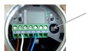
Connection plug for the MPI-200-F adapter as an intermediate plug between the ILM-4 electronics and the MPI-200 connection 3 (see the next figure).
